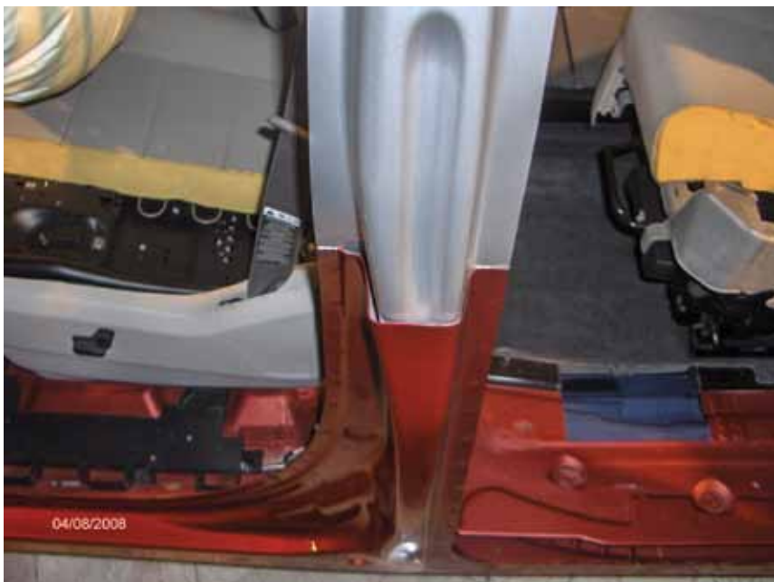
The cut-away view of the B-pillar in this demonstration vehicle reveals that the B-pillar is not entirely Boron steel. Only the silver-colored inner layer of steel shown here is Boron. In most cases, only one layer of two or three layers will be advanced steel. In the real-world, there is no visible difference between the appearance of normal mild steel and any of the advanced steels on a vehicle.
